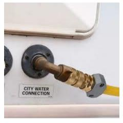
Fill line to non-portable tank with a quick disconnect coupler
