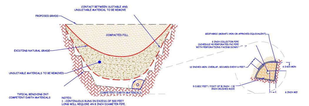
2 - FINAL 20 FEET OF PIPE AT OUTLET WILL BE SOLID AND BACKFILLED WITH COMPACTED FINE-GRAINED EARTH MATERIALS.
