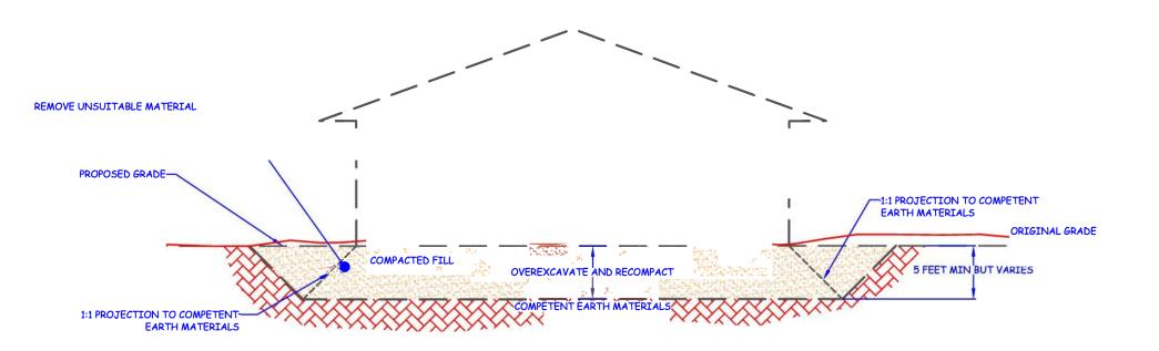
NOTE; REMOVAL BOTTOMS SHOULD BE GRADED WITH A MINIMUM 2% FALL TOWARDS STREET OR OTHER SUITABLE AREA (AS DETERMINED BY THE GEOTECHNICAL CONSULTANT) TO AVOID PONDING BELOW THE BUILDING
