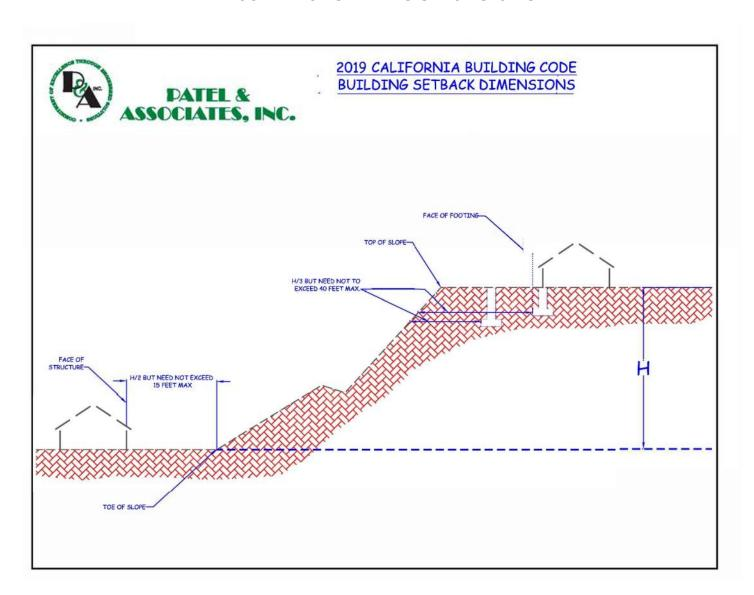
When determining the required clearance from ascending slopes with a retaining wall at the toe, the height of the slope shall be measured from the top of the wall to the top of the slope.
