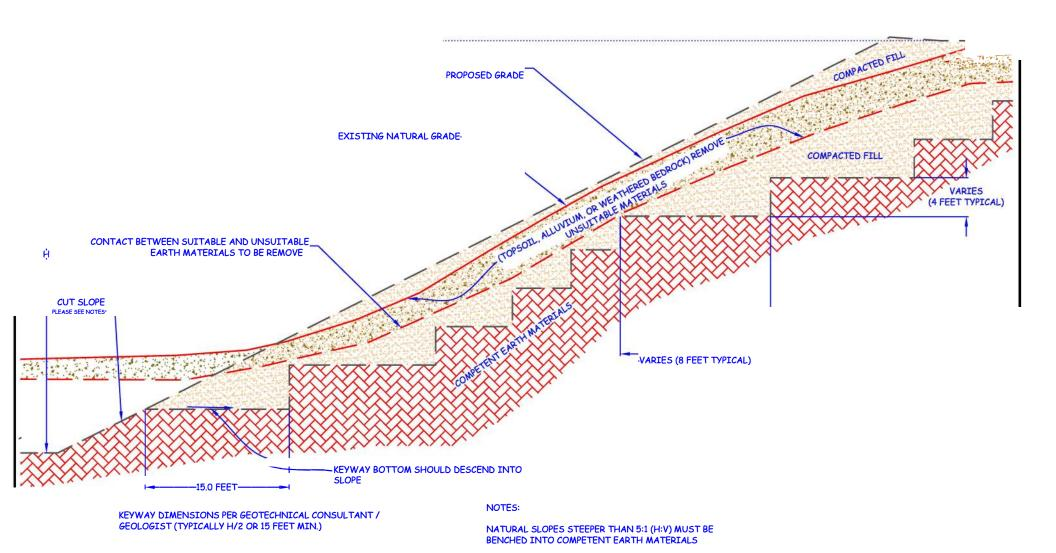
THE CUT SLOPE MUST BE CONSTRUCTED FIRST
