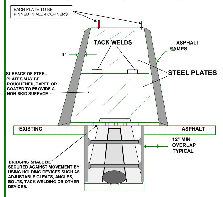
NOTE: TRENCH WALLS AND ADJACENT SOIL SHALL BE SUFFICIENTLY STABLE FOR THE USE OF THE ABOVE PLATE.
