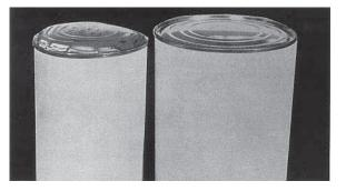
Gas formation in can which causes one or both ends to swell producing a flipper, soft swell, hard swell, or blown can. Hold for investigation.
