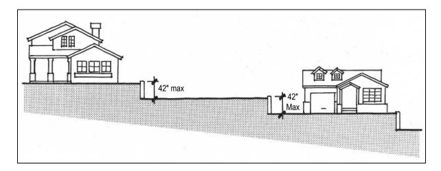
Figure 83-11 Retaining Walls for Side Setbacks
