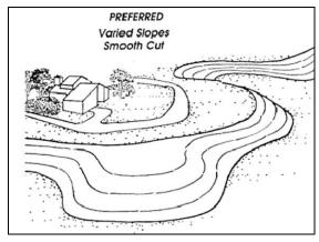
Figure 83-9 Variations in Cut and/or Fill Slopes
