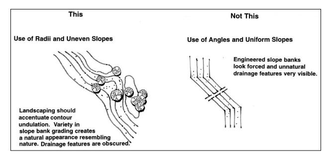
Figure 83-7 Characteristics of Manufactured Slopes
