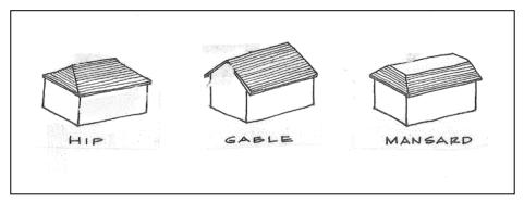
Figure 84-14 Typical Roof Types
