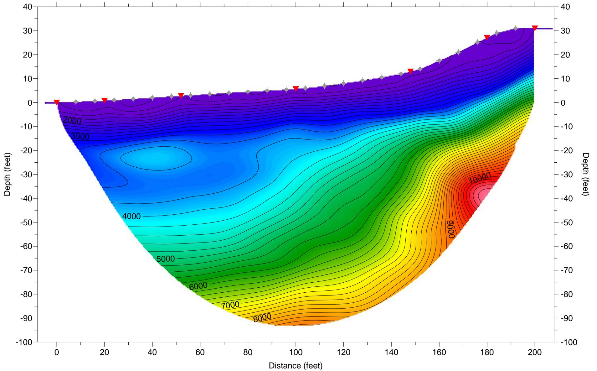
SEISMIC LINE S-1, 20 WET iterations, RMS error 1.0 %, DeltatV initial model artefacts !, Version 3.31
