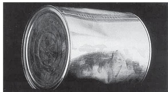
**3** Paneled non-beaded can. Materially affecting appearance, but not integrity, no plate fractures.
