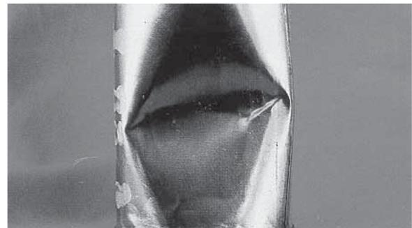
**2** Severe body dent. Observe for fractured plate.
