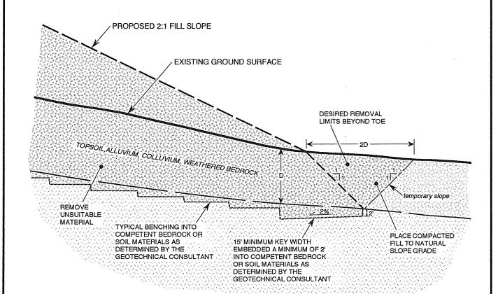
D = RECOMMENDED DEPTH OF REMOVAL PER GEOTECHNICAL REPORT
