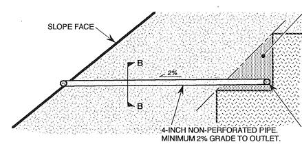
APPROVED FILTER MATERIAL (OPEN-GRADED GRAVEL WRAPPED IN FILTER FABRIC OR CLASS 2 FILTER MATERIAL).
