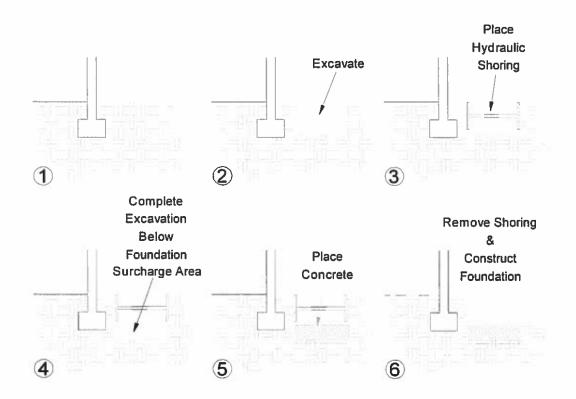
7.21.2 It is recommended that an equivalent fluid pressure based on the table below, be utilized for design of hydraulic shoring.
