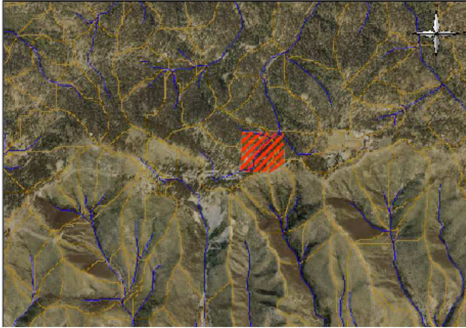
Figure 3: Watershed basins fall away to the North and to the South of the projected site. The site itself drains Northeast into Daley Canyon. (Watershed basins are delimited by orange lines, and major drainage lines are in blue.)
