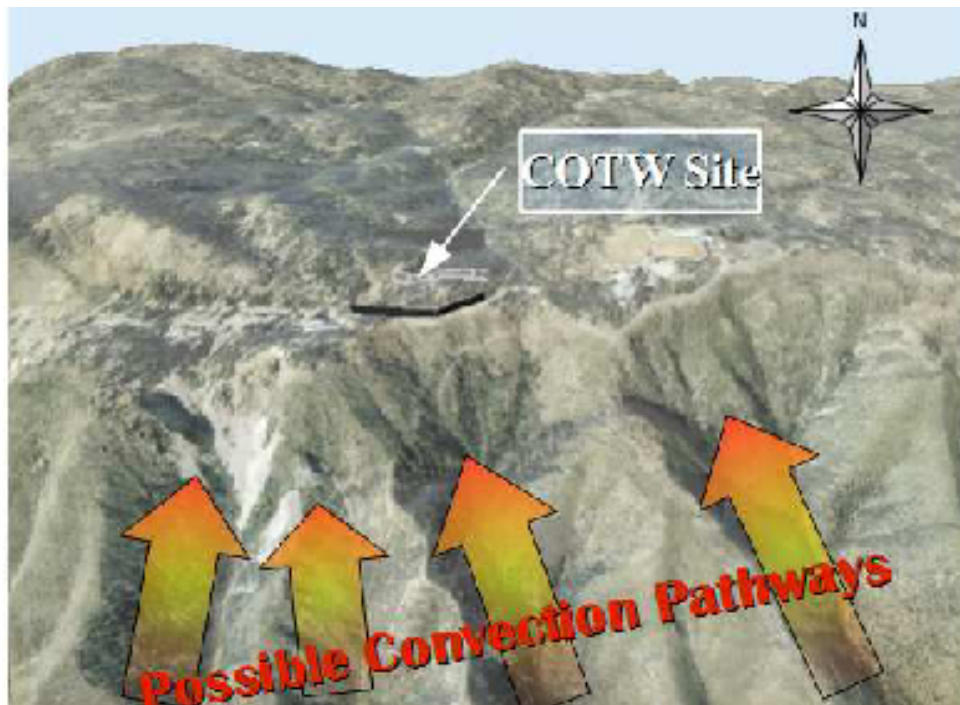
Figure 11: The location of the COTW site can make it particularly susceptible to effects of southerly winds, 'chimney' effects of convection up the drainages to the South, and in these same drainages, the potential for the development of local inversions that can burst causing an instantaneous 'flash' effect due to combustible gases that were trapped under the inversion layer.
