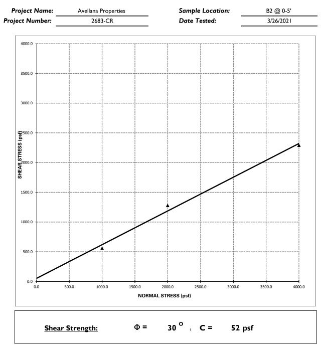
**Notes:** I - The soil specimen used in the shear box was a ring sample remolded to approximately 90% relative compaction from a bulk sample collected during the field investigation.
