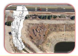
This project is the long term, permanent solution to the recharge limitations at the Turner Basins. The turnout will be approximately 200 linear feet of 16 inch steel pipe and supply 10 cubic feet per second of water to the basins.
