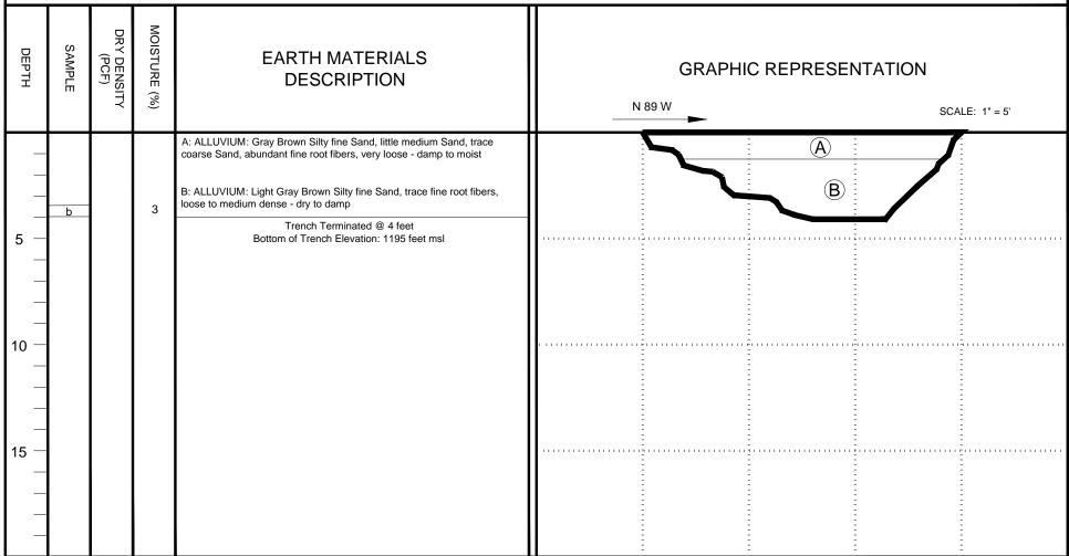
KEY TO SAMPLE TYPES: B - BULK SAMPLE (DISTURBED) R - RING SAMPLE 2-1/2" DIAMETER (RELATIVELY UNDISTURBED)
