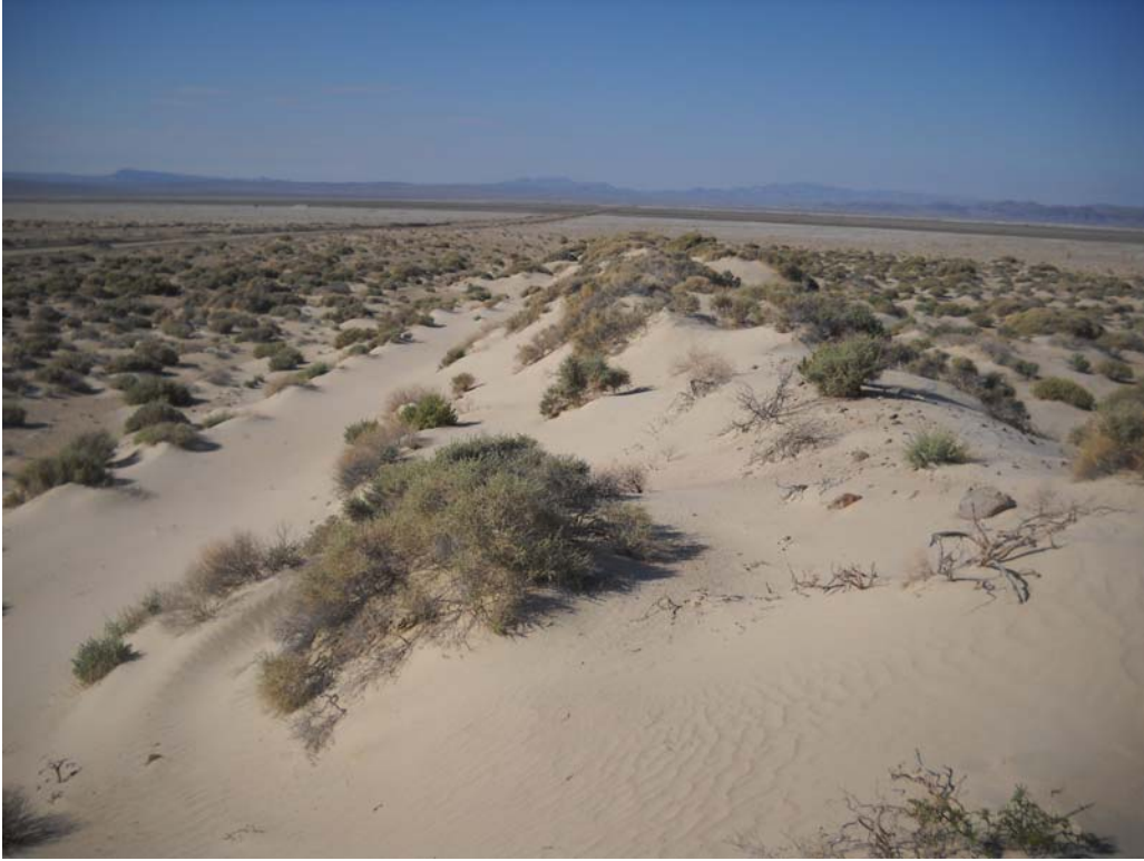
Photo No. 7. – Unsuitable material (eolian sand) within the “Zone-of-Influence”.
