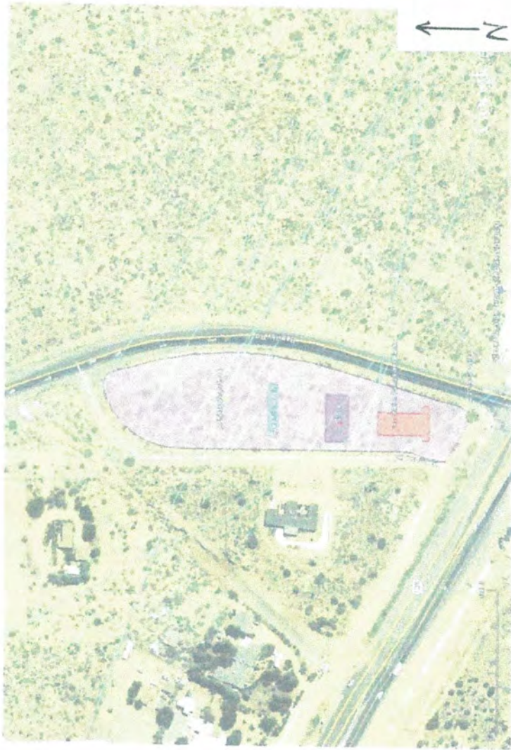
P201700597, APN 3066 191-04 showing proposed store and gasoline pumps and tanks wrt suspected faults (blue lines)
