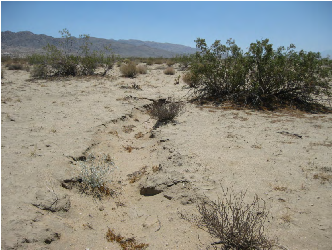
Photo 17: Offsite channel exhibits typical crust on soil surface and loose conditions where soil has been disturbed.
