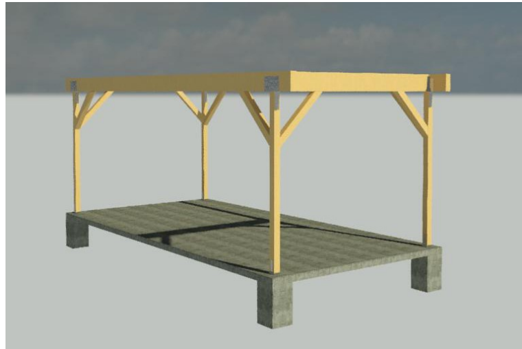
COLUMNS AND BEAMS CONSTRUCTED WITH HARDWARE IN PLACE
