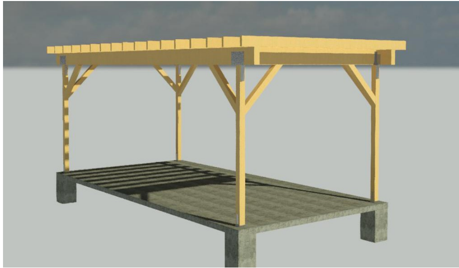
ROOF JOISTS INSTALLED
