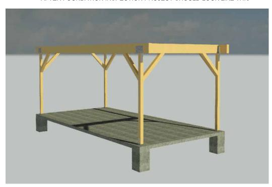
COLUMNS AND BEAMS CONSTUCTED WITH HARDWARE IN PLACE
