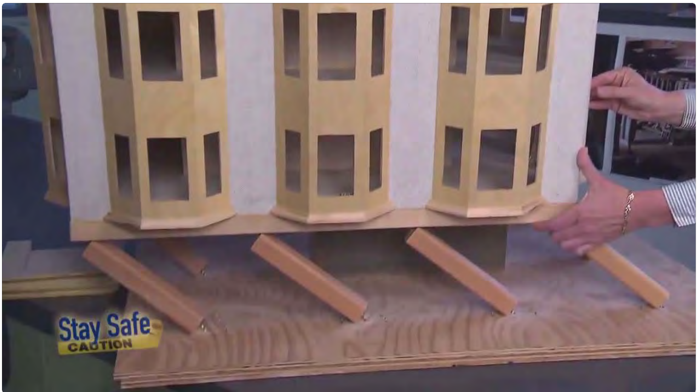
A model of how a wooden apartment complex with carport parking on the first story, held up by flimsy columns, can collapse. Source: SFGovTV
