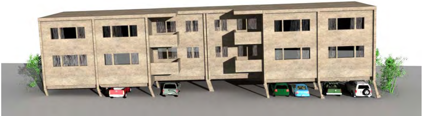
Why wood apartments can collapse in earthquakes (Raoul Ranoa / Los Angeles Times)
